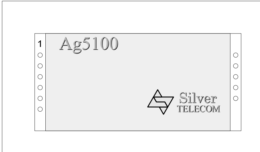
Figure 2: Ag5100 DIL Package Format (Top View)
